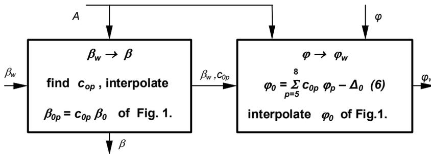
Fig. 6. The scheme of INT  $\beta, \varphi$  program.
