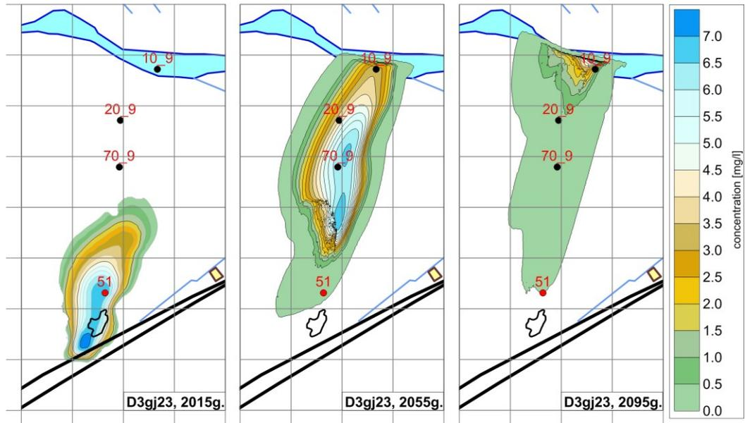
Figure 6. The Northern plume (no decay) in 2015, 2055 and 2095
