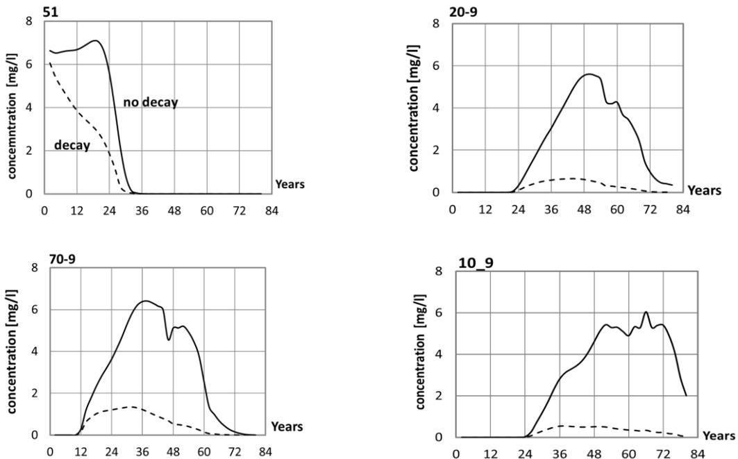
Figure 7. The SAS concentration [mg/l] for monitoring wells Nos 51, 70-9, 20-9, 10-9 of the SAS no decay and decay cases
