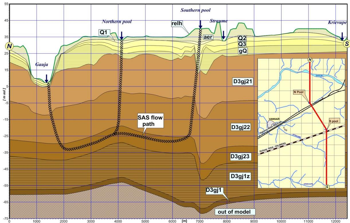
Figure 3. Cross section N-S; SAS plumes are located within the subaquifer D3gj23.
